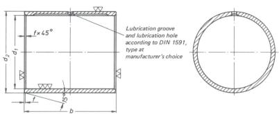
Designation of a bearing bush with bore  $d_1 = 90 \text{ mm}$ :
