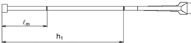
Figure 13: Marking lengths l_m on extension pipe for injection of adhesive
