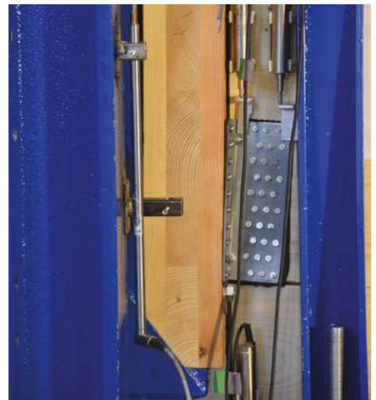
Test samples: CLT panels TITAN TTF200 angle bracket
