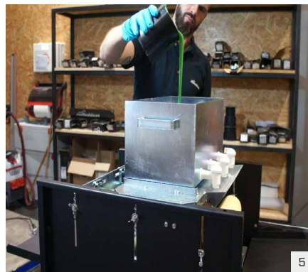
5 Enter paint or impregnating primer. If necessary, mix it until a homogeneous consistency is obtained.
