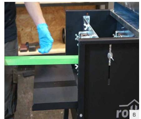
6 Start the process: open the nozzles and wait for the rolls to absorb the colour. Finally, push the elements through the sponges.
