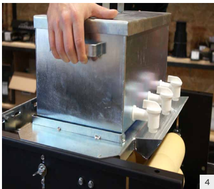
4 Position the colour tank and make sure that nozzles are closed. Hook the collection bucket under the tank.
